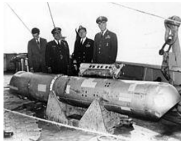
The B28RI nuclear bomb, recovered from 2,850 feet (870 m) of water, on the deck of the USS Petrel.
